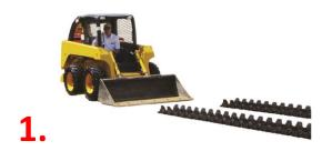
1. Make sure that both tracks are parallel to each other and of equal distance to the machine. Remove as much slack as possible.
