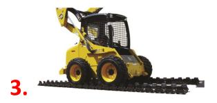
3. Slowly drive the machine over the tracks. Stop halfway over the track chain.
