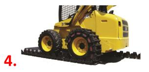
4. Fold the back end of tracks over the back tire of the machine.
