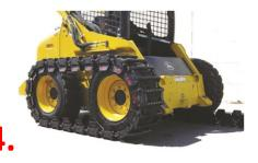
14. Remove the installation tool from the track and then move the machine forward until there is an open space to insert the carriage bolt on the inside of the track. Tighten the bolt.
