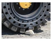
backhoes don't use an axle mounted suspension, they are vulnerable to vibrations from the ground, which makes Nu-Air's superior shock-absorption an even more welcoming feature. Add to this the zero chance to ever get flats, and you got an undisputed winner."
