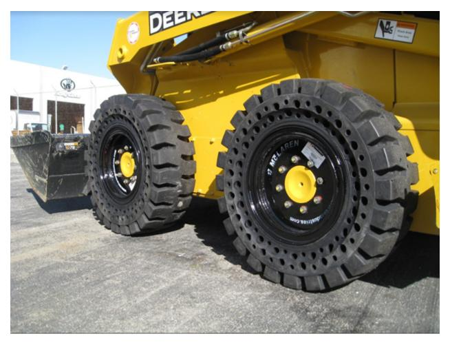
When choosing a solid or flat-proof tire, one of the largest concerns is typically how much cushion or shock absorption the tire offers. Since skid steers don't have a suspension system like a car would, the tire *becomes* the suspension. As such, if a tire is solid and hard, the skid steer operator would feel every little bump in the road which would create a highly uncomfortable ride, among other issues.
