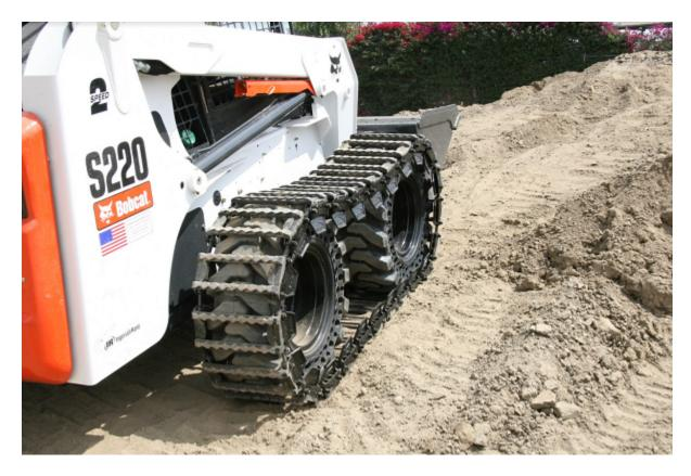
One of the best upgrades that you can get for a skid steer loader with tires is **over-the-tire skid steer tracks**. From expanding the capabilities of your machine to increasing its revenue potential, there are numerous advantages that these versatile tracks offer. To learn about some of the most impactful benefits of over-the-tire skid steer tracks, continue reading.
