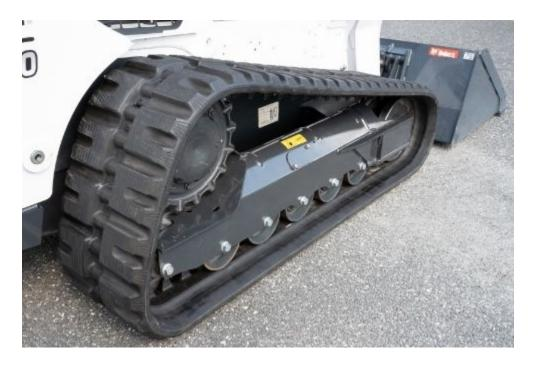
Inside of a <u>rubber track</u>, a steel cable is what gives the track its tensile strength. Without this wire, you could pull on the track, and it would stretch—similar to how a rubber band would. However, these steel wires inside the rubber track prevent it from stretching out. Ultimately, there are two ways to implement steel cables inside a track. Below, we'll address some of the key differences between continuous wound vs. overlapping connections on rubber tracks.
