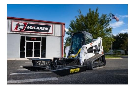
Brush cutter attachments are an ideal option for efficiently cutting through thick overgrowth that would typically destroy a standard mower. If your application could benefit from one of these durable attachments, you have two main options to choose from: a gear-driven brush cutter or a direct drive brush cutter. To determine which option will best suit your application, check out these tips on how to choose a brush cutter.
