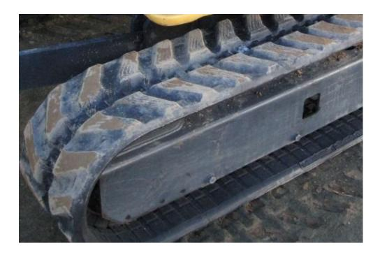
Compact track loaders are staples for many construction and landscaping companies. These important pieces of heavy machinery feature ultra-durable, high-flotation rubber tracks that allow them to traverse delicate surfaces and poor ground conditions.
